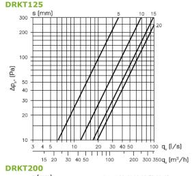
s (mm) 10 15 20 25 30 35 40 300 200 100 (Pa) 50 Δp., 40 30 20 10 100 200 300 q, (l/s) 56 10 20 30 40 50 100 ..... Т Т Т 20 30 40 50 100 200 300 500 1000 q, (m³/h)
