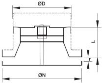
The valve is closed when the inner disc of the valve actuating element coincides with the zero-plane, Fig. Actuating valve element has only positive travel; it is totally opened when actuating valve element is moved 25 mm from the zero plane. For one turn of the valve actuating element it is longitudinally displaced for 1 mm. The graphic shows the dependence of flow rate, noise intensity and total pressure drop across the valve type DVSR100 and DVSR125.
